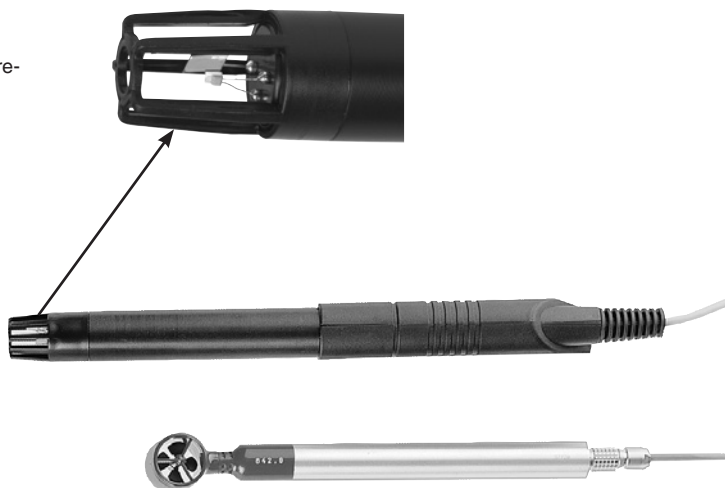
Fig. top: combined temperature-humidity probe
