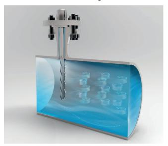
The helical coils, arranged around the thermowell stem of the ScrutonWell® design, break up the flow and thus impede the formation of a clearly defined Kármán vortex street. Through the reduced amplitudes of the diffused vortices, vibrational excitation of the thermowell is avoided.
