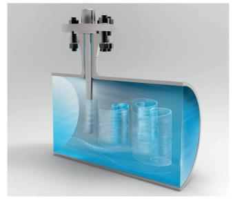
In certain flow conditions, a Kármán vortex street can form behind the thermowell stem when it is subjected to a flow within a pipeline. This vortex street consists of two rows of vortices with opposite directions of rotation, which detach themselves to the left and the right of the thermowell out of phase, and this can instigate the thermowell to vibrate.
